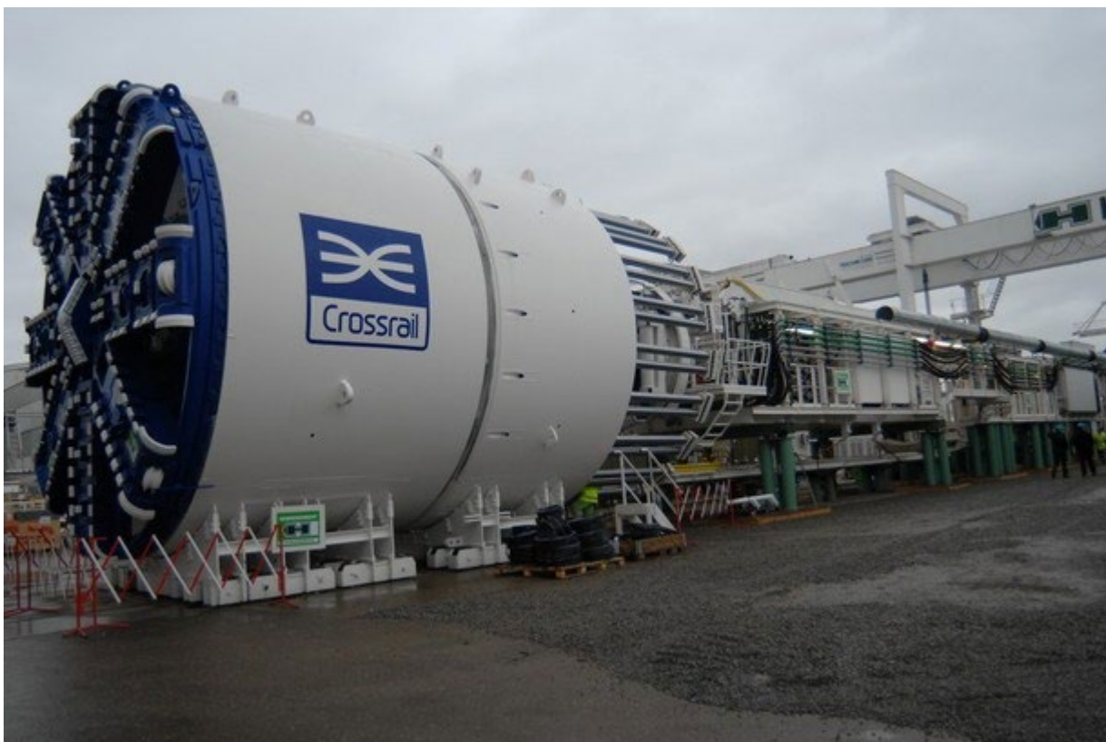
Figure C7: ~Crossrail 7.1m diameter Earth Pressure Balance TBM (© Herrenknecht)
