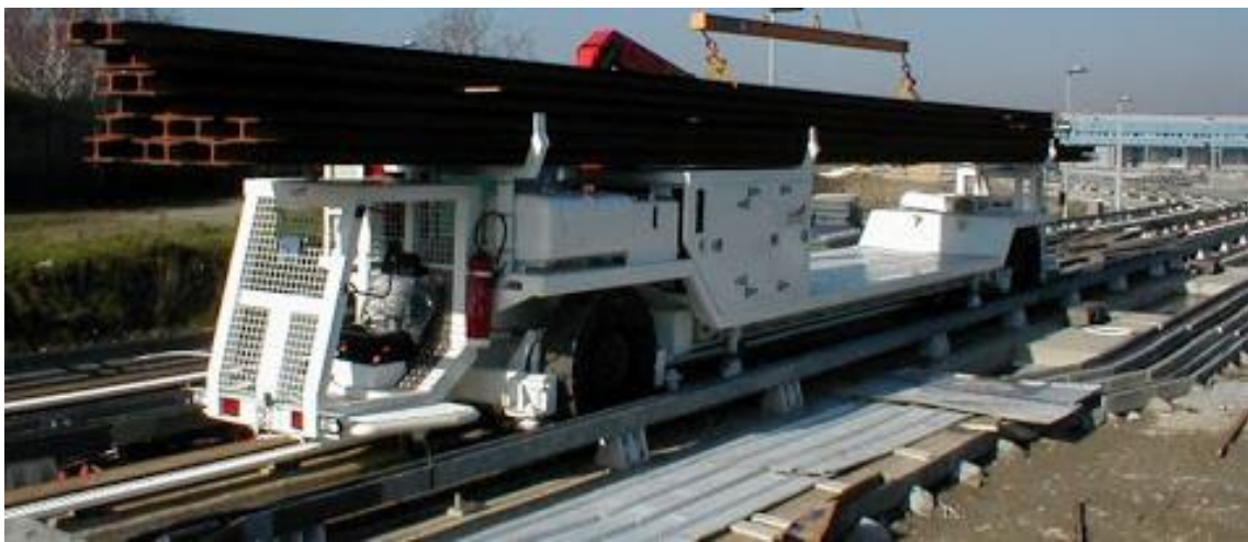
Figure C15: MSV with captive rail guidance and rack & pinion
