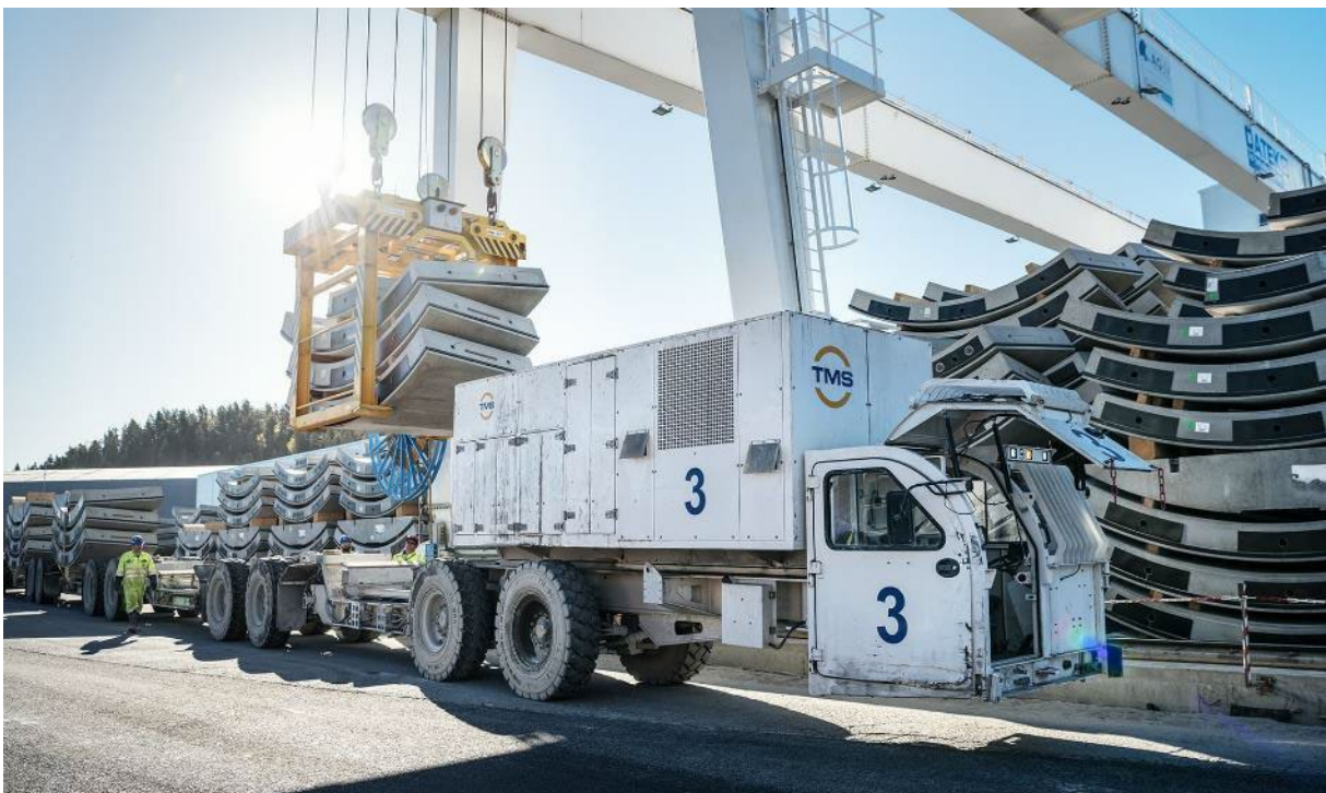
Figure C13: Concrete tunnel segment loading onto an MSV (© TMS)
