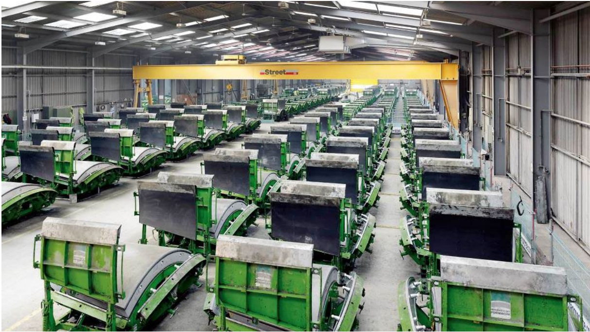
Figure C12: Segment factory with casting moulds (© Herrenknecht)
