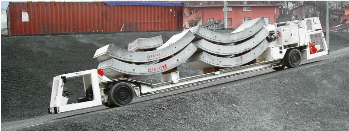
Figure C14: Dual cab MSV operating on an incline with concrete segments
